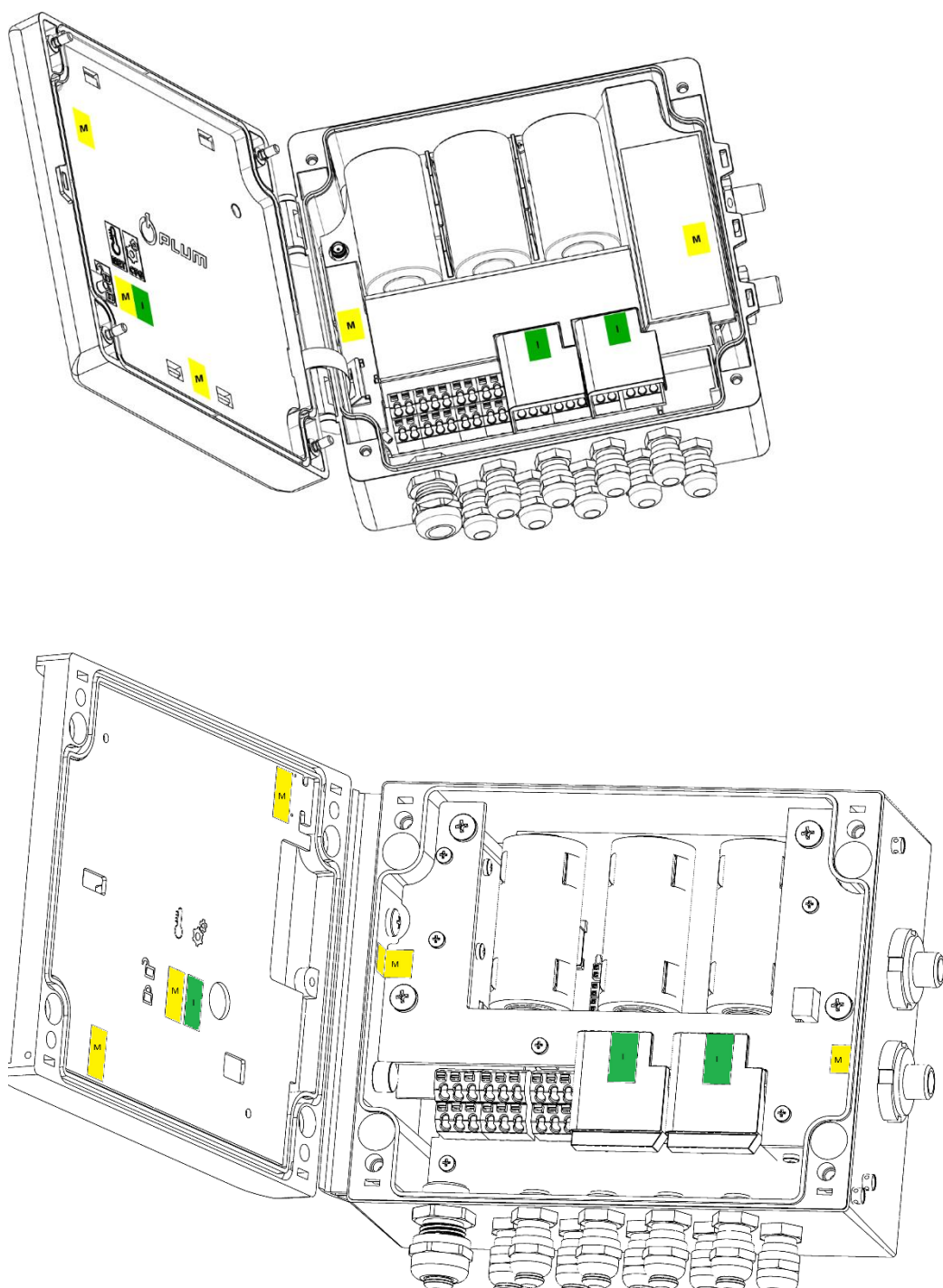
Figure 6. Internal sealing of MacBAT 5: M – sealing mark, I – installer seal
